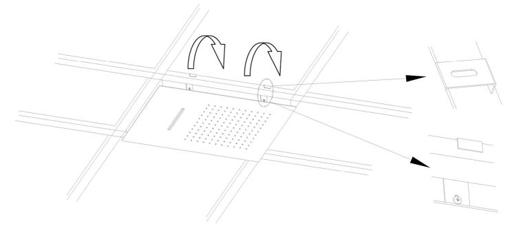
Step 4 The fitting base of shower head should hang on and connect water inlet, Then finished
