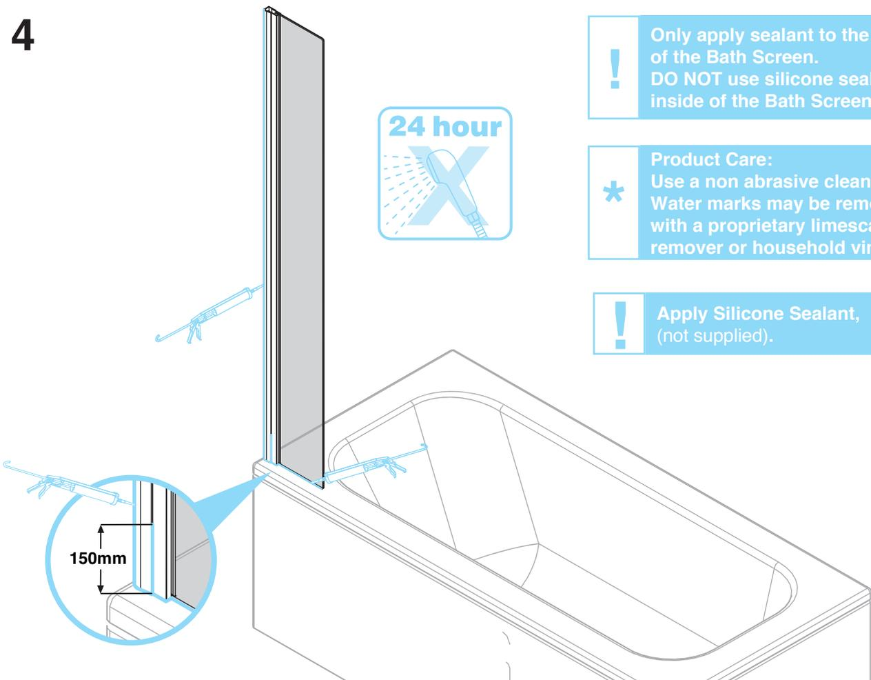
**!** Only apply sealant to the outside of the Bath Screen. DO NOT use silicone sealant on inside of the Bath Screen.
