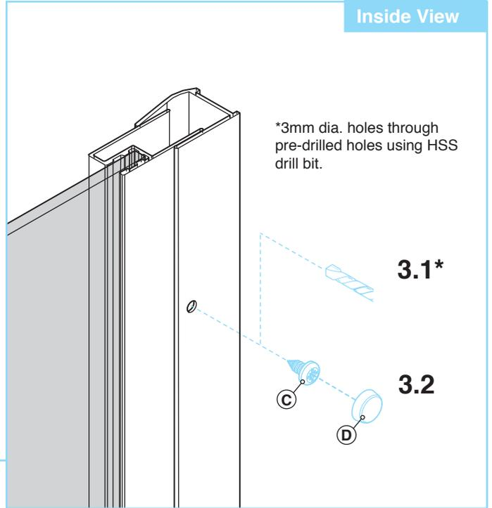
**!** Ensure Bath Screen is level prior to fixing, adjust to suit.
