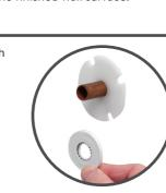
im the projecting pipe to a length of 15-22mm, measured from the face of the gripper ring, using a suitable cutter. If a hacksaw is used, the pipe end must be carefully de-burred and chamfered.
