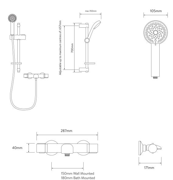
\*Pipe centres can be adjusted between 130mm-170mm using supplied elbows
