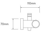
\*Pipe centres can be adjusted between 130mm-170mm using supplied elbows
