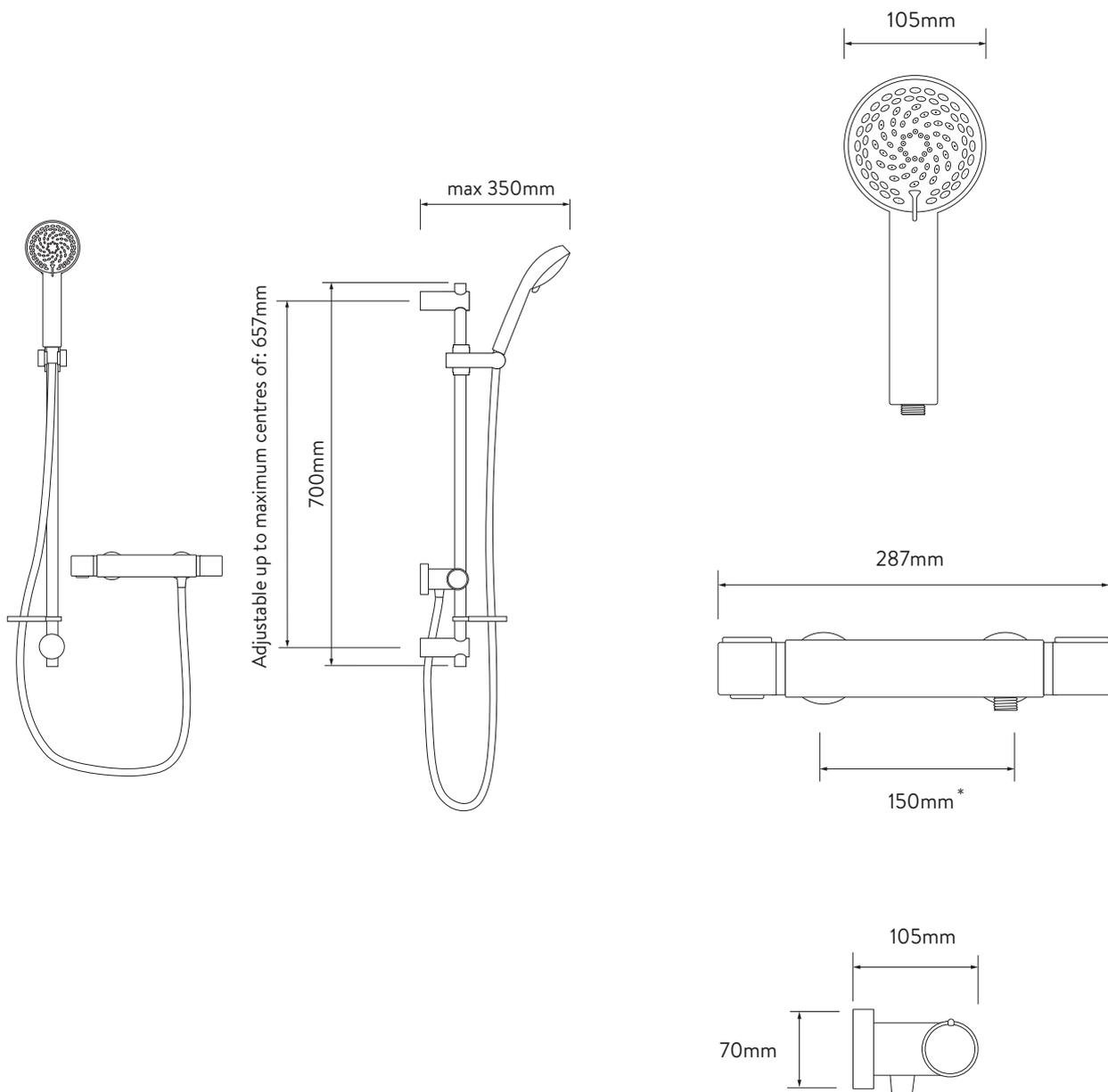
\*Pipe centres can be adjusted between 130mm-170mm using supplied elbows
