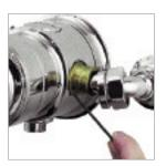
Place the assembly into the mounting ring and onto the supply pipes. Tighten the locking screw to secure the assembly to the mounting ring using the 2.5mm hexagonal key provided.
