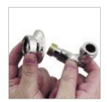
Carefully slide the dummy nuts onto the elbows ensuring damage to the plated surfaces is avoided.
