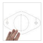
Remove the mounting ring from the rear of the valve using the 2.5mm hexagonal key provided. Locate the ring inside the pre marked position, ensuring the locking screw is in the 6 o'clock position and mark the four fixing holes.
