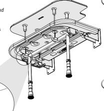
To fit retainer, it should be rotated in a clockwise direction whilst applying firm pressure towards the seat.
