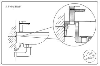
Place the basin over the screws and use the plastic bushing and nut to tighten into place. Tighten evenly by hand and finish off with a spanner.
