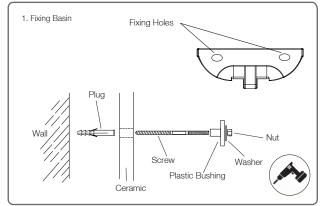
Ensure the wall is strong enough to support the basin and semi pedestal. Hold the basin up to test and ensure optimum height (recomended 800-850mm from tap deck to floor). Make sure the semi pedestal will cover the pipework when placed over and then mark out and drill the holes for the basin. The plugs and screws can then be inserted and tightened with a spanner.
