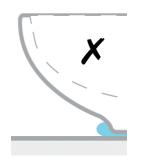
Apply the silicone slightly in from the edge of the outer edge of the underside of the basin
