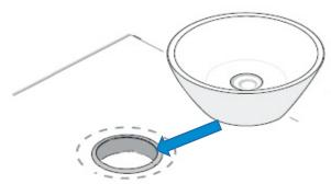
Place the basin into position with the waste through the drilled hole Allow all sealant to dry for at least 24 hours before use
