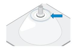
Cut holes if necessary for waste and tap ensuring the tap hole is positioned at a distance which does not cause interference with the basin Seal the inside/exposed edge after cutting to prevent water/moisture penetration
