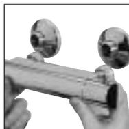
**9** Attach the hose to the valve hose outlet to allow the water to discharge safely to waste. Turn on the supplies to the shower and turn the shower on to flush the system through. Turn off the shower.
