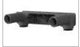
**1** Eccentric elbows are provided to allow for inlet pipework adjustment between 140mm – 160mm centres. Construct suitable connections terminating in ½" BSP female fittings.
