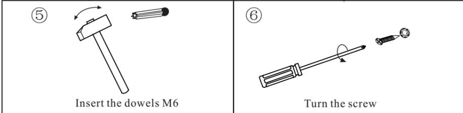
⑤. Insert the dowels into the drilled hole with hammer.
