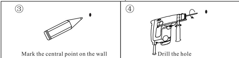
③. Determine the position of two central points on the wall with tape at the installation position, and then mark with pencil.
