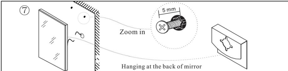
⑦. Keep the power off and connect the wires of the mirror to the wires exposed on wall. Hang the mirror to the screws.
