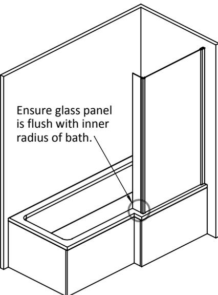
Slide the wall profile (2) onto the screen. Sit the screen onto the bath and adjust so the short glass panel butts up to the inside radius of the bath. Mark the position of the wall profile (2) with a pencil.
