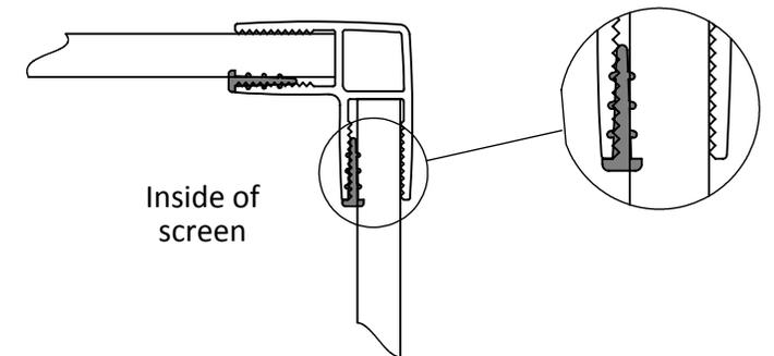
Insert the vertical wedge seal (6) into the corner post as shown above. Push the seal down the length of the corner post. A wooden block can be used to aid fitting. Trim off any surplus seal at either end, so its level with the profile.
