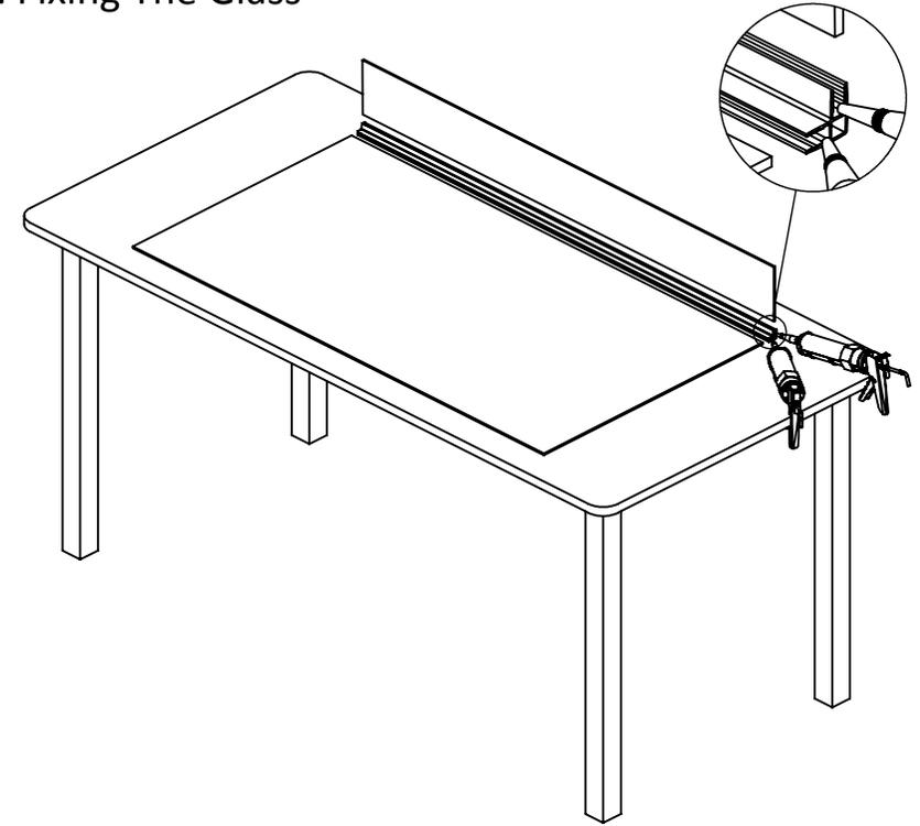
Lay the large panel (4) on a clean flat surface with the corner post (1) facing upwards. In both corner post slots, apply a small bead of silicone along the length of the channel stopping 5mm short of either end and insert the glass panels (4&5).
