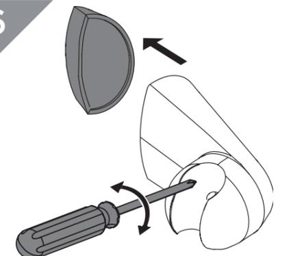
Push the wall bracket onto the fixing bracket, you will hear a 'click' once secure. The handset holder can be adjusted to suit.
