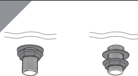
Secure the body to the bath by using the washer and metal backnut below the bath. Tighten the backnut onto the threaded tails.
