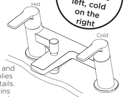
Connect the hot and cold water supplies to the threaded tails. Turn on the mains water supply and check connections for any leaks.
