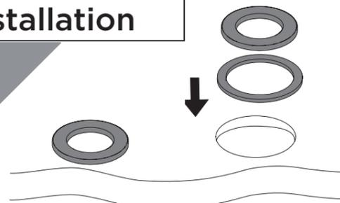
Place the plinths over the holes in the bath ensuring that the washers are fitted between the plinths and the bath.
