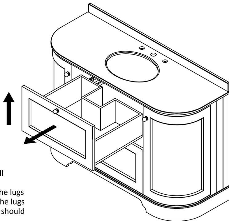
To remove drawer from cabinet, pull-out the drawer to it's full extension and gently lift the drawer box upwards.
